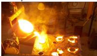
Stage 10: Metal is poured into the inert ceramic mould. Emissions reduced due to absence of a resin binder in the sand.
