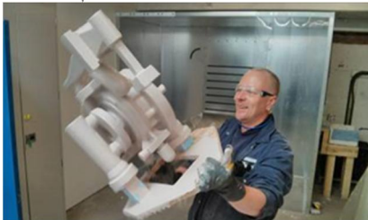
Stage 4: Coat polystyrene pattern with ceramic slurry and backup
