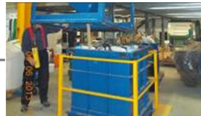
Stage 8: Ceramic shell assemblies are packed into a casing box with
