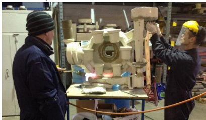
Stage 7: Ceramic sub assemblies can be joined together.
