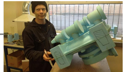
Stage 3: Assemble and wax component for improved surface finish.
